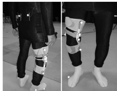
Fig.7 The position of marker attached for structure analysis of knee-orthosis.
