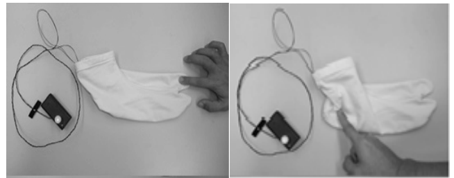
Fig.4 Footswitches of the heel and the toe.
